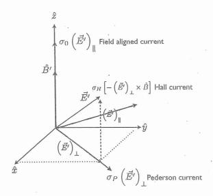
Ionospheric current equation:  $J = \sigma \cdot (E + U \times B)$
