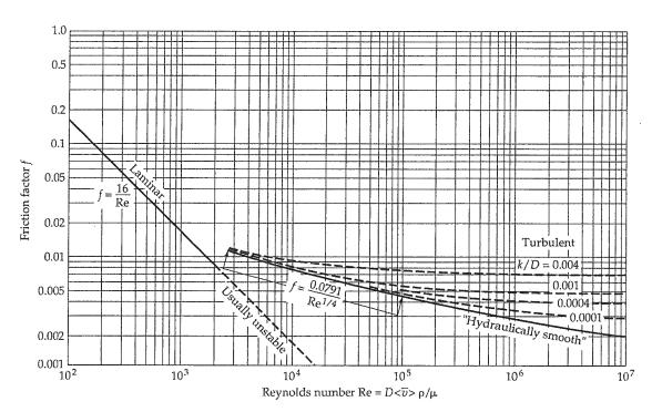
$$\text{Laminar: } f = \frac{16}{\text{Re}} \quad \text{Re < 2100}$$
