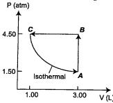
shown in figure. The CA process is a reversible isothermal expansion. What is (a) the net work done by the gas during one cycle? (3%) (b) How much energy is added to the gas by heat during on cycle? (3%) (c) How much energy is exhausted from the gas by heat during one cycle? (3%) (d) What is efficiency of the cycle? (3%)
