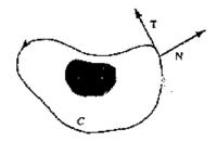
region D. At any point on C, let T be the unit tangential vector in the positive direction and N the unit outer normal vector. Assume velocity vector V is known in region D, except the shaded area. Find a method to compute divergence of V integrated over region D. That is,
