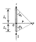
Show that the magnetic field of flux intensity  $\vec{B}$  at point P (distance r from axis) in the figure is given by  $\vec{B} = \vec{a}_{\phi} \frac{\mu_0 I}{4\pi r} (\cos \alpha_1 + \cos \alpha_2)$  (T). (10%)
