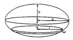
Figure 1 The Earth is an ellipsoidal shape whose equatorial radius  $r_e$  is slightly greater than its polar radius  $r_p$ . A thin disc is shown which is parallel to the equator, has a radius r and thickness  $\Delta z$  and is a vertical distance z from the equator.
