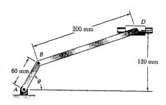
4. The uniform slender rod AB is in equilibrium in the position shown when end A is given a slight nudge, causing the rod to rotate counterclockwise and hit the horizontal surface. Knowing that the coefficient of restitution between the knob at A and the horizontal surface is 0.40, determine the maximum angle of rebound  $\theta$  of the rod. (20  $\Re$ )
