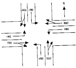
S (TH+RT) = 1800 (vehicles/hour) for through and right turn movement S (LT) = \$00 (vehicles/hour) for permitted left turn movement
