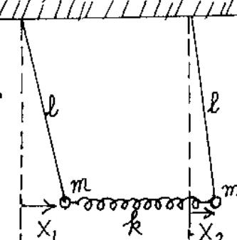
We select as coordinates  $x_1$  and  $x_2$ , measured positively to the right from the equilibrium positions of the two masses. (The length of the string in each case is  $l$ , and the mass of the bob in each case is  $m$ .) Write the equations of motion for small displacements in terms of the coordinates  $x_1$  and  $x_2$  and other parameters.
