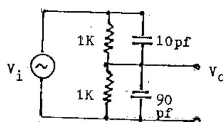
3. In the circuit as shown. Assume the input pulse is wide enough to allow completion of the circuit response to the leading edge of the pulse. Find the output waveform. ( 20% )
