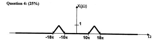
An analogous signal x(t) has the Fourier transform indicated in the figure. The signal is sampled to obtain the discrete time signal
